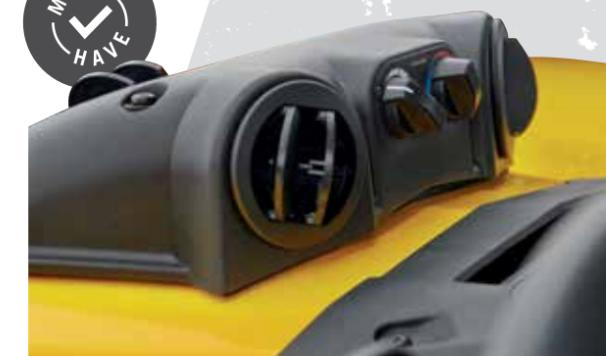
**BEST INTEGRATED SYSTEM ON THE MARKET WITH 6 VENTS, 3 FAN SPEEDS AND IN-DASH ADJUSTABLE TEMPERATURE FOR ULTIMATE WINDSHIELD DEFROSTING/DEICING AND FOOT-HAND HEAT.**
