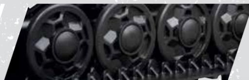
Rubber over molded heavy-duty double bearing wheels and offset wheel spacing reduce friction and vibration while ensuring reliability.
